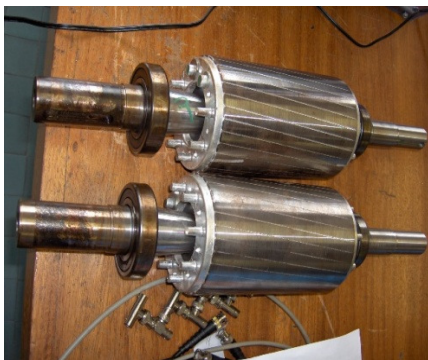
Fig. 3: Accelerated wear of the bearings by immersion in acid
